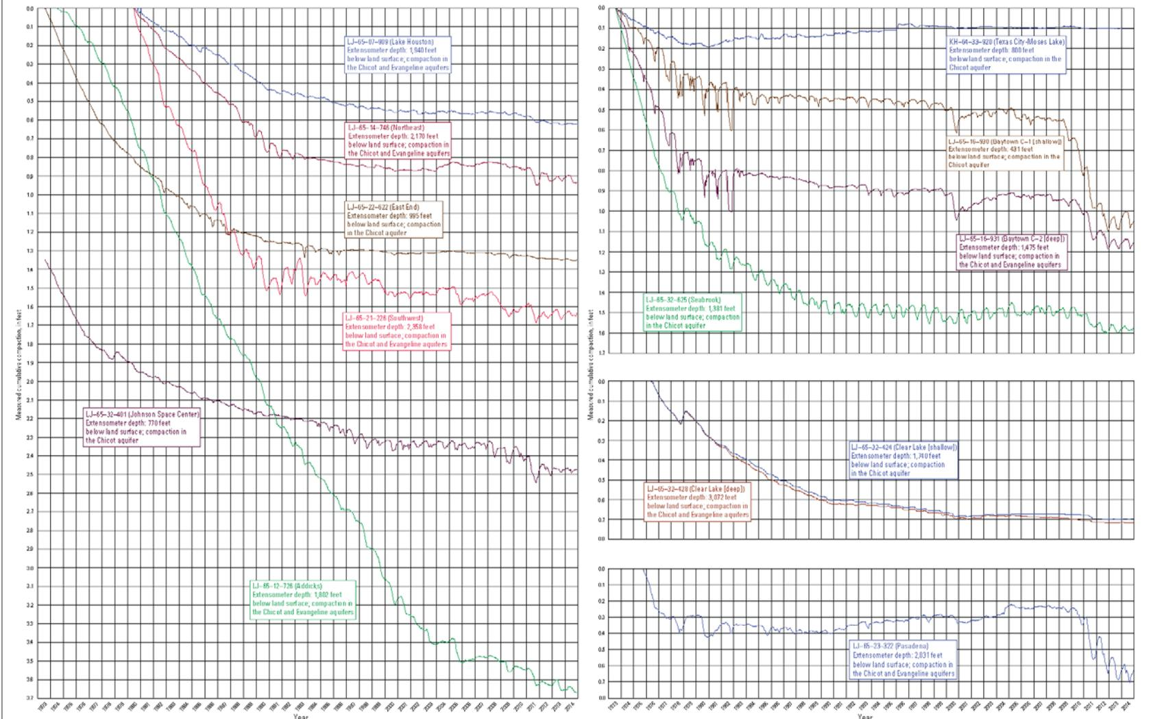
Sheet 16. Measured cumulative compaction of subsurface sediments at borehole-estensometer sites depicted on sheet 15, 1973–2014.
